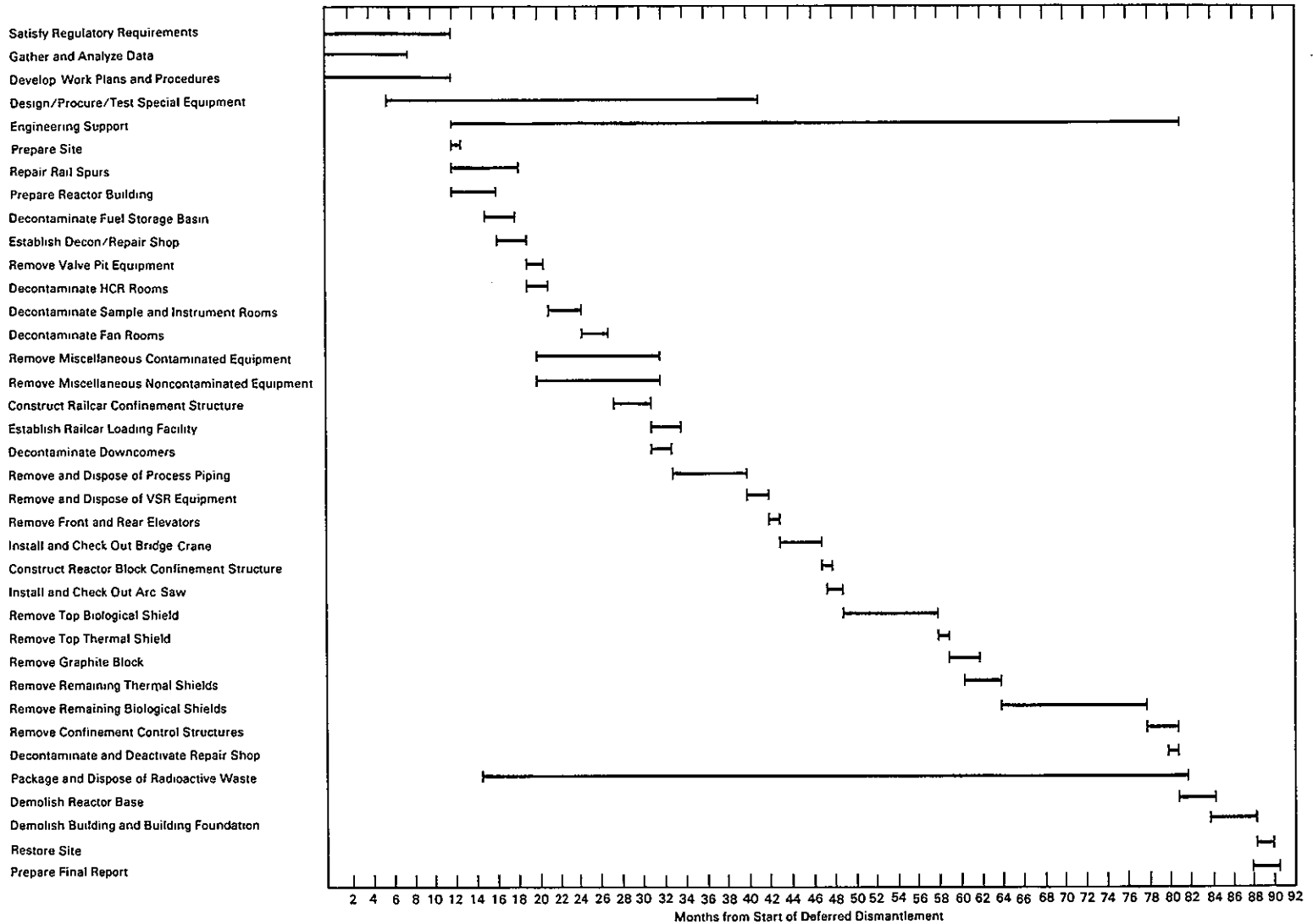
FIGURE 3.7. Deferred Dismantlement Schedule for a Single Reactor
